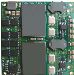
1/2 Brick 70A Output 2.4 x 2.28 x 0.45 (in) 60.9 x 57.9 x 11.4 (mm)
