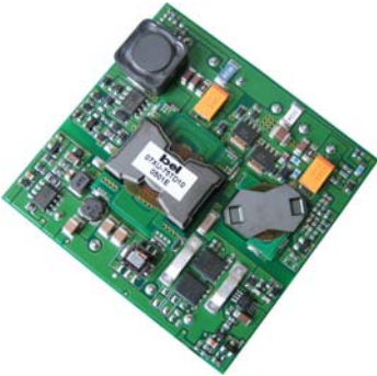
07XU-75TD10 78W Output 2.4 x 2.28 x 0.48 (in) 60.9 x 57.9 x 12.2 (mm)
