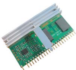
xRPG SIP Series 30 / 40A Output 2.4 x 1.25 x 0.5 (in) 58.8 x 30.6 x 12.3 (mm)
