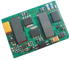
1/16 Brick Series 5A - 25A Output 1.3 x 0.9 x 0.35 (in) 33.0 x 22.9 x 8.9 (mm)
