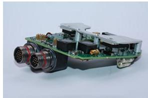
The customized connectors set (Male + Female) was strictly designed with a special mechanical shape to be located at accurate match inside the payload slip ring system. The contact arrangement was specially designed for a customer requierments and contains 32 contacts for data (size 22), 4 contacts for power lines (size 20) and one MMCX coaxial contact for the video link. The connectors are Hermetically Sealed to 10-5 cc/sec Helium level..
